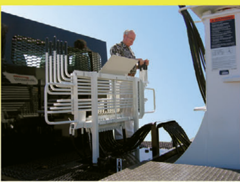
Standard dual walk-thru controls shorten cycle times
